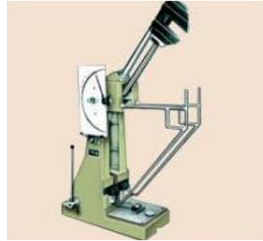
Impact (Charpy Izod ) testing machine
