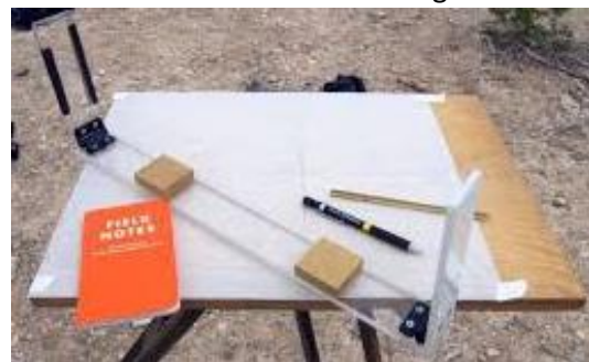
Plane table surveying
